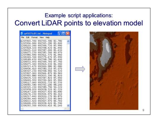
Scripts can convert data among different formats. In this case, the script uses point coordinate information in a text file to create a Digital Elevation Model. The advantage of the script in this case is that it can automatically process the hundreds or thousands of individual files that comprise certain high-resolution remote sensing datasets.
